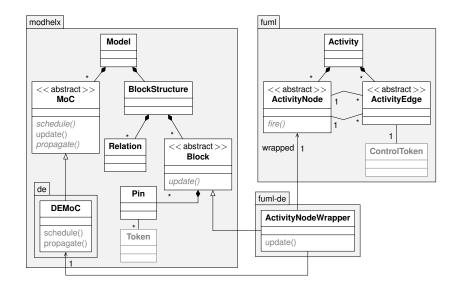
**Fig. 8.** Mapping (package fuml-de) between the kermeta-based implementation of fUML (package fuml) and ModHel'X (package modhelx) to use any of its MoCs (*e.g.*, here the discrete event MoC, package de)
